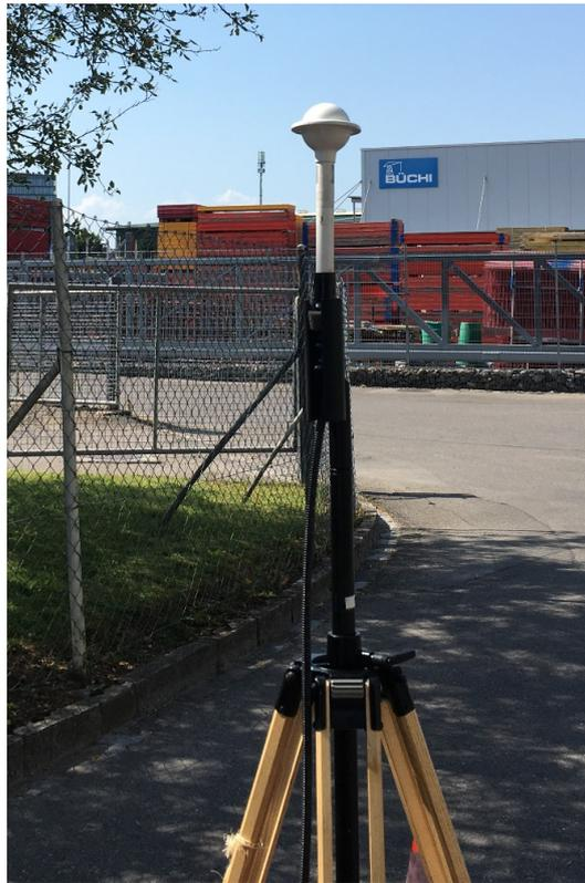
**Figure 1.** Tri-axial Satimo INSITE Free electric-field probe (at a height of 1.5 m) in line-of-sight of a fifth generation new radio base station in Bern, Switzerland.
